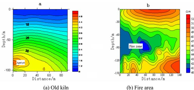
Figure 4. TEM detection profile of the goaf and fire zone in Xinjiang.
