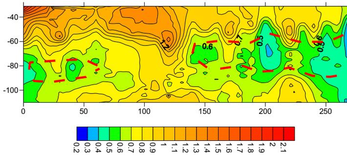
Figure 7. TEM apparent resistivity profile of a coal mine tunnel side.
