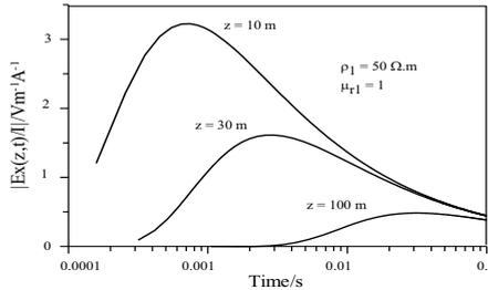
Figure 1. Transient responses of a step pulse at various distances ( $\rho_1 = 50 \Omega\cdot\text{m}$ ,  $\mu_{r1} = 1$ ,  $\epsilon_{r1} = 15$ ).
