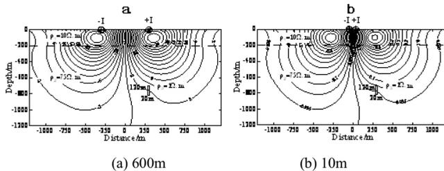
Figure 2. Transient electric contour for different size loops.
