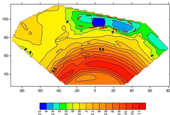
**Figure 8.** TEM apparent resistivity profile of a coal mine tunnel ahead.
