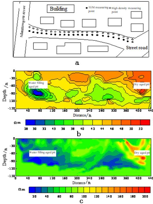
(a) Construction layout; (b) Apparent resistivity-apparent depth profile of high density electrical method; (c) TEM apparent resistivity-apparent depth profile
