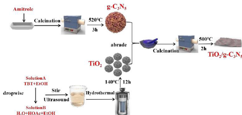
Figure 3. Flow chart of composite photocatalytic material preparation.
