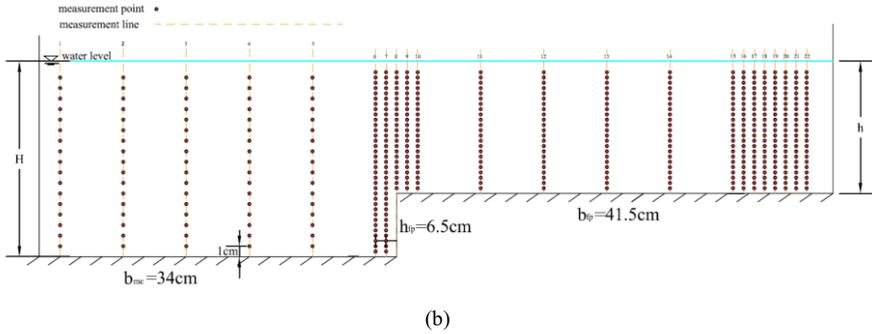
Figure 2. (a) Vegetation arrangement in a plan view and (b) measurement points.
