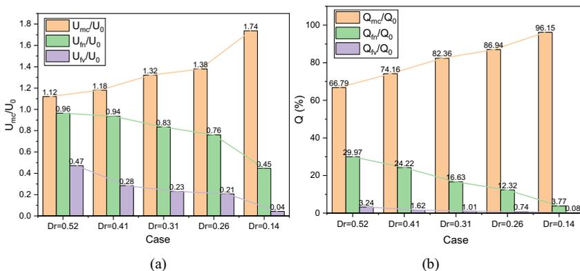
Figure 3. (a) The dimensionless zonal velocity and (b) The ratio of the zonal discharge to the total discharge in percentage.
