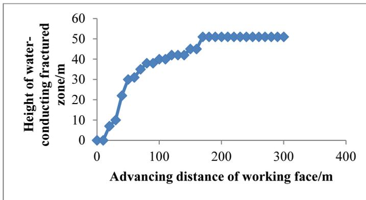
Figure 2. Height development curve of water conducting fractured zone with 1-2 coal seam mining.
