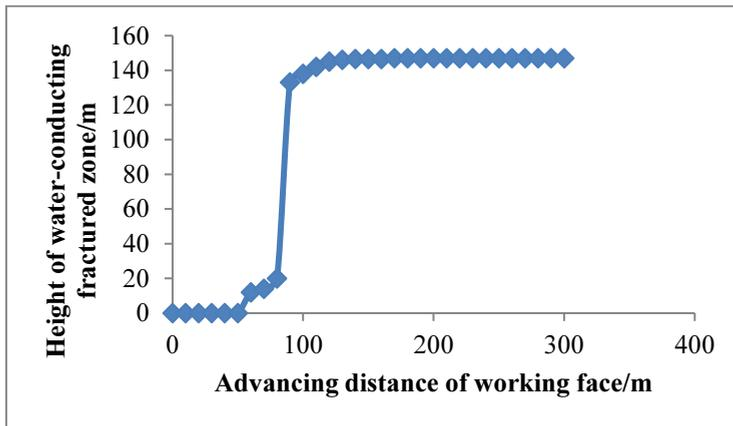
Figure 3. Height development curve of water conducting fractured zone with 2-2 coal seam mining.
