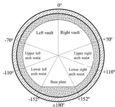
Figure 11. Numbering diagram.
