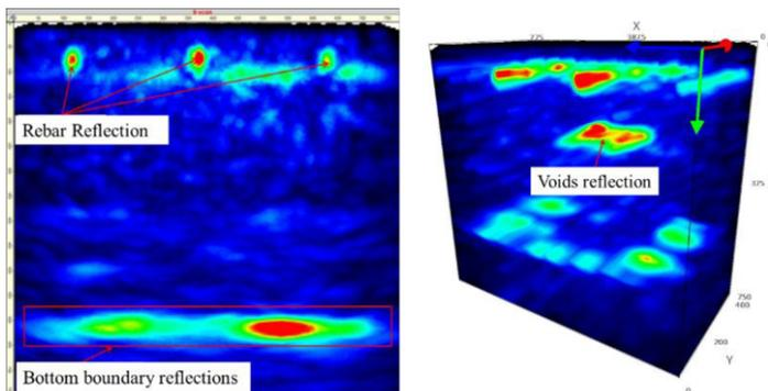
Figure 9. Ultrasonic Tomography Technology results.
