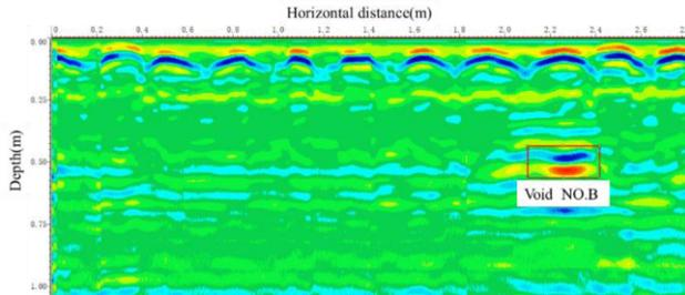
**Figure 7.** Ground-Penetrating Radar results.
