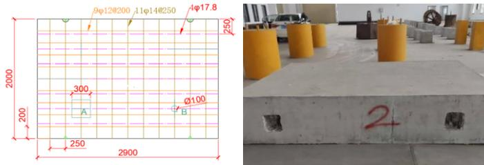
Figure 6. The lining model.
