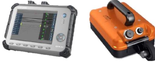
**Figure 2.** Ground Penetrating Radar (GPR) equipment.
