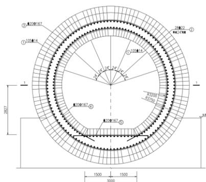
Figure 1. Hydraulic tunnel cross-sections.
