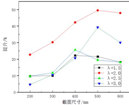
Figure 4. Influence of size on reinforcement effect of steel strip.
