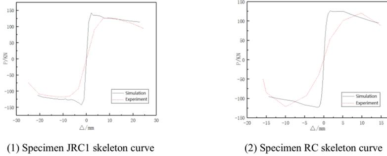
Figure 2. RC and JRC1 simulation and test comparison.
