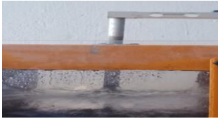
Figure 3. Jet striking vane.
