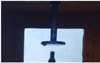
Figure 5. Jet and Vane arrangement.
