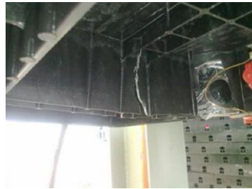
(c) Cracked template next to handle.
