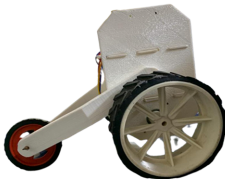
Fig 14. The final chassis and trailing arm assembly with a total printing time of 26 hours with a 20% infill of the PLA+ filament with a 0.4 mm nozzle.
