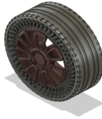
Figure 2. 3D model of NPT Tweel 12N16.5.
