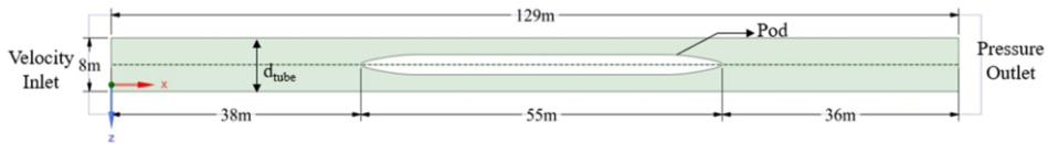
Figure 1. Geometry of hyperloop pod inside a tube
