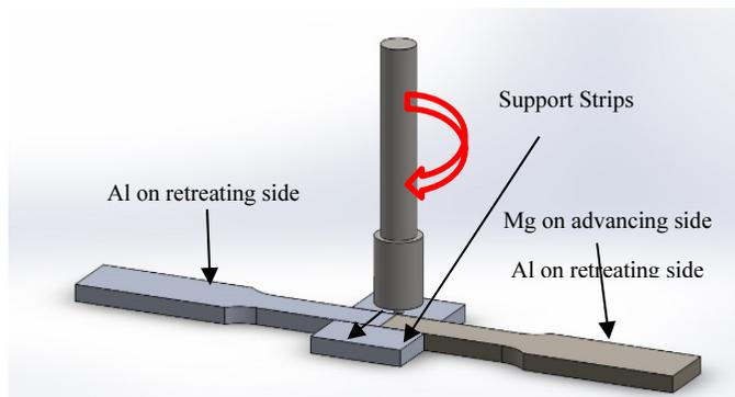
Figure 1. FSW Setup
