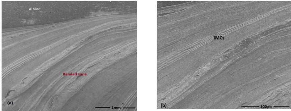
**Figure 2.** SEM of Weld Zone Showing Intermixing of Both Metals
