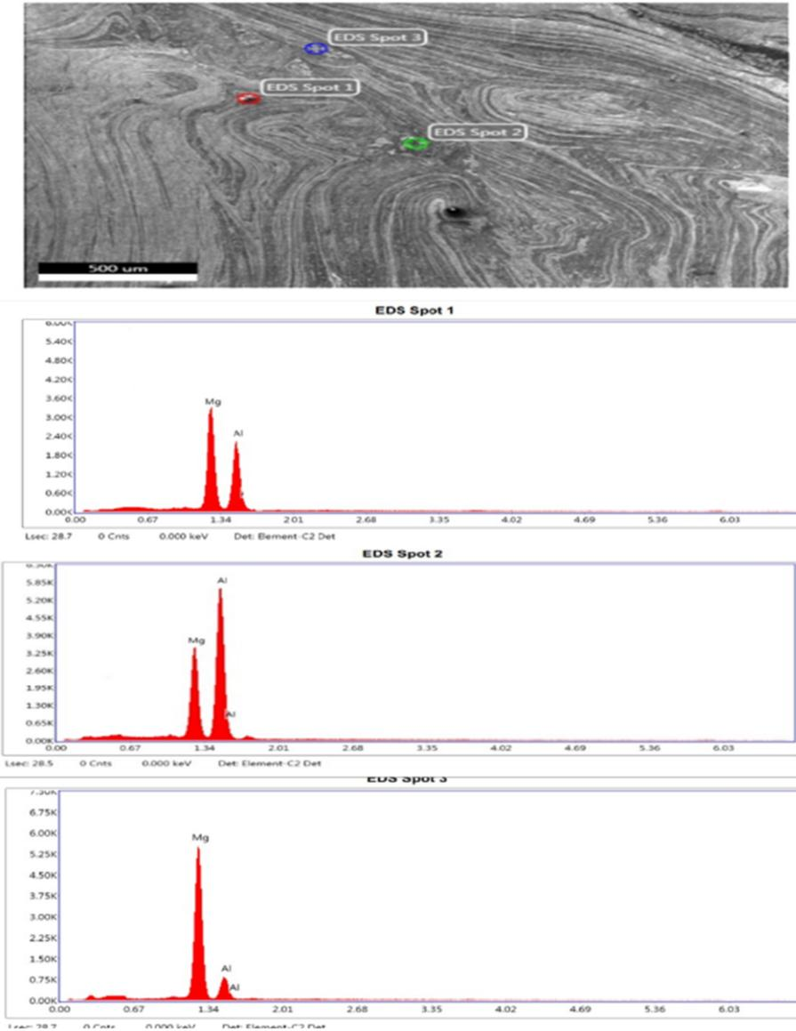
**Figure 4.** EDX Spectroscopy, Composition Graphs
