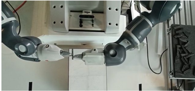
Figure 4. Top view of the robot transferring a piece from its left hand to its right hand, to turn it over and place it correctly on the plate. The plate can be seen below the robot's hands. On the righthand side of the image, the bin-picking station contains multiple pieces in random positions, ready to be processed,
