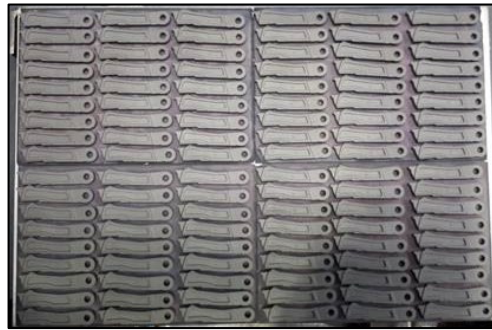
Figure 2. Example of a reference (L·W·D = 46·10·5 mm approx.). 108 pieces arranged on a 6x18 matrix pattern, on a plate with dimensions (approximate) 206x305mm. No physical contact between pieces.
