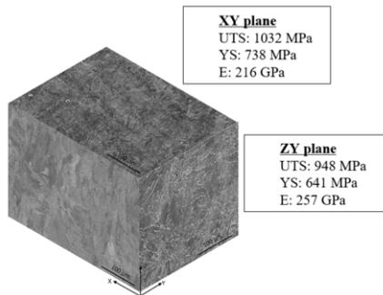
**Figure 1.** Scanning Electron Microscopic image of LPBF IN718 built in XY, YX and ZX direction with the UTS, YS and young modulus, E of the XY and ZX samples
