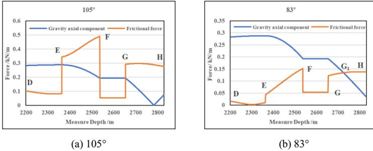
Figure 5. Axial force component for target section deviation 105° and 83°
