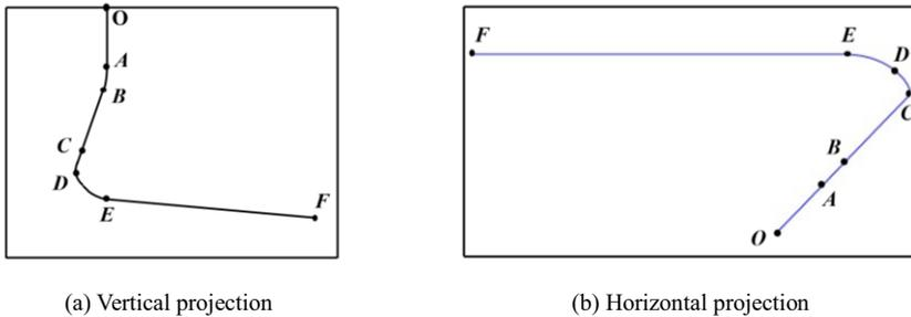
Figure 1. Well trajectory of a spoon-shaped well.
