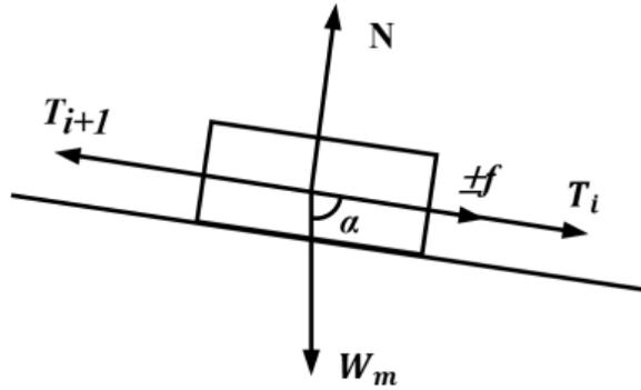
Figure 2. Force analysis of string element in slant section.
