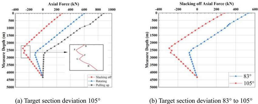
Figure 4. Effect of target section deviation on string axial forces.
