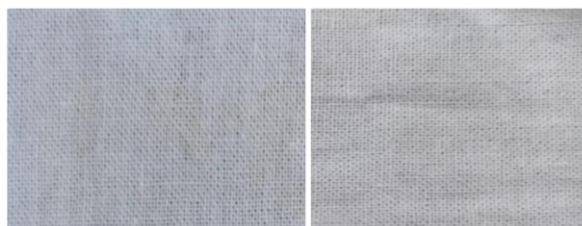
Figure 4. The electrochemical dyeing (left) and traditional dyeing cloth sample (right).
