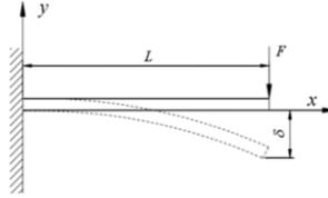
Figure 4. Cantilever beam structural mechanics model.
