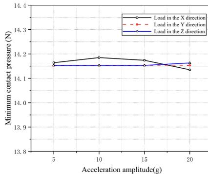
**Figure 7.** Minimum contact pressure under different acceleration amplitudes.
