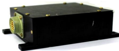
Figure 2. Appearance of a three-component magnetometer installed on board a pilot model of the Aist small spacecraft.
