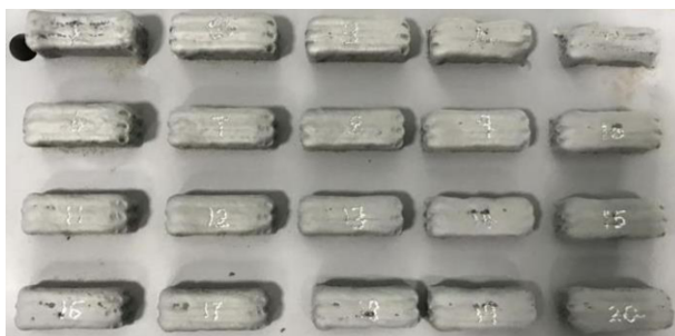
Figure 1. Inconel 718 alloy block with different Nb contents manufactured by the high-throughput 3D-printing.
