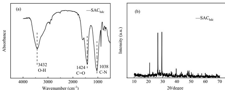
Figure 3. (a): FT-IR spectra; (b): XRD patterns.
