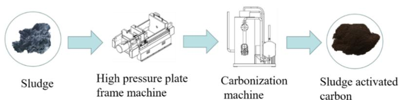
Figure 1. Flow chart of SAC<sub>hdc</sub> preparation.
