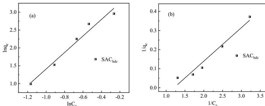
**Figure 6.** (a): Freundlich adsorption isotherm; (b): Langmuir adsorption isotherm.
