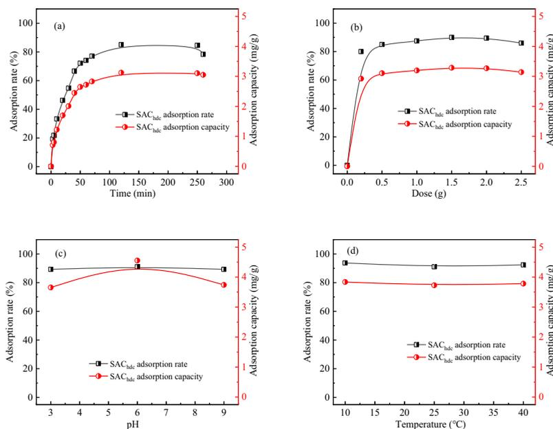
Figure 4. (a): The effects of time on the adsorption; (b): The effects of dose on the adsorption; (c) The effects of pH on the adsorption; (d): The effects of temperature on the adsorption.
