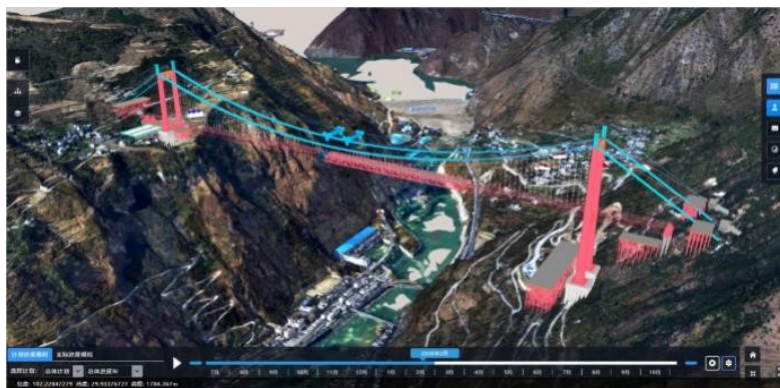
Figure 6. 4D construction simulation based on virtual construction platform.
