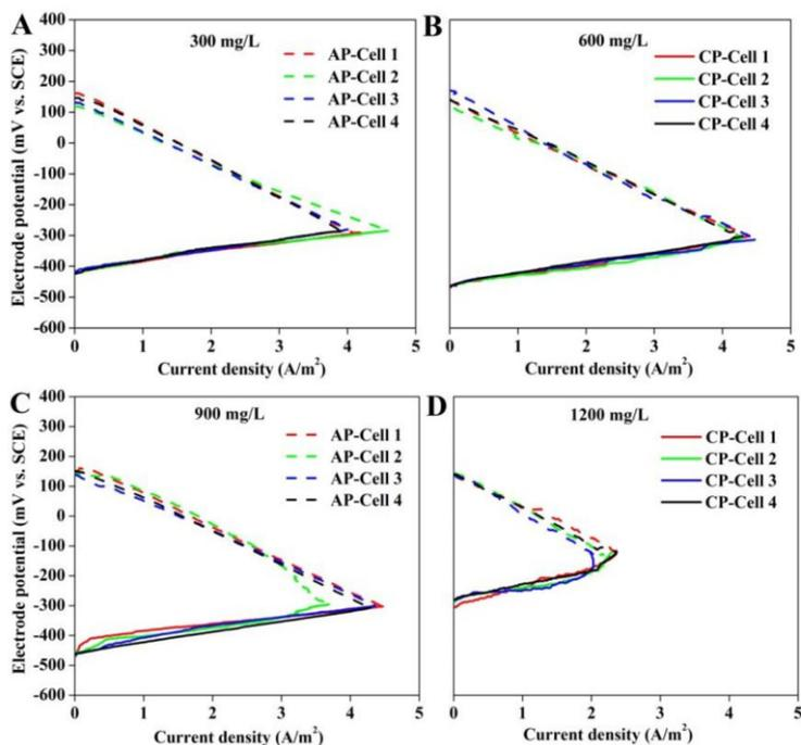
**Figure 4.** Electrode potentials of the CSBES at different ammonia concentrations. (a): 300 mg/L; (b): 600 mg/L; (c): 900 mg/L; (d): 1200 mg/L.
