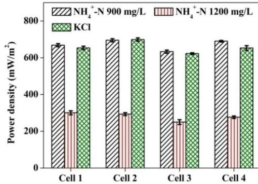
Figure 7. The maximum power densities of CSBES under NH<sub>4</sub>Cl and KCl conditions.
