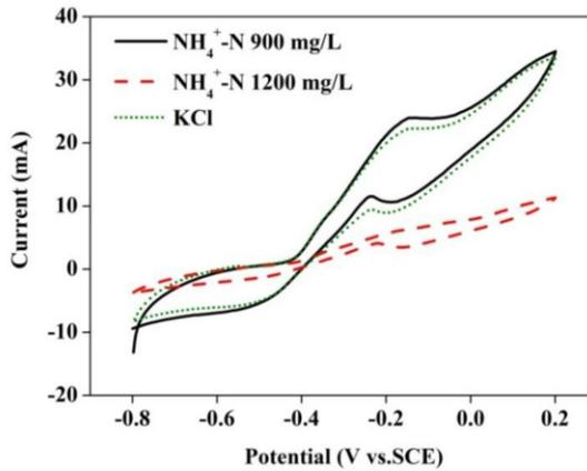
Figure 8. Cyclic voltammogram of anode biofilm (Cell 1) under NH<sub>4</sub>Cl and KCl conditions.
