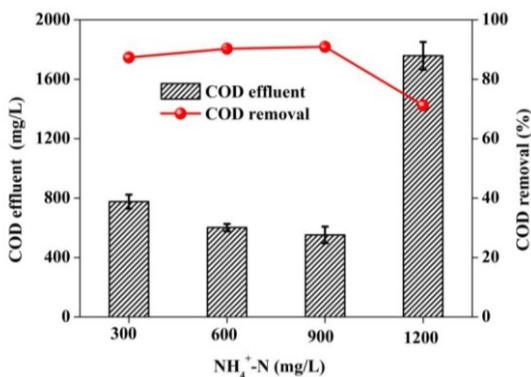
Figure 5. Effluent COD and COD removal in CSBES at different ammonia concentrations.
