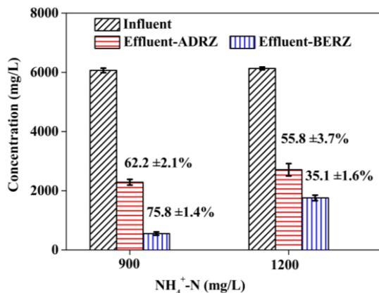
Figure 6. Effluent COD of ADRZ and BERZ at ammonia concentration of 900 mg/L and 1200 mg/L.
