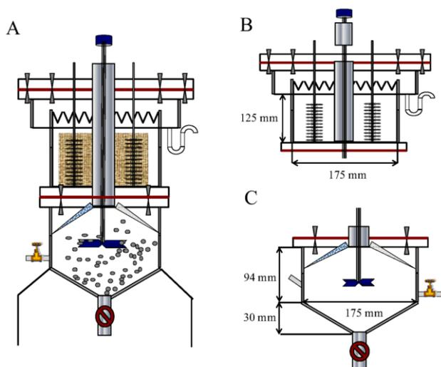
**Figure 1.** (a) The continuous stirred bioelectrochemical system (CSBES); (b) Bioelectrochemical reaction zone (BERZ); (c) anaerobic digestion reaction zone (ADRZ).
