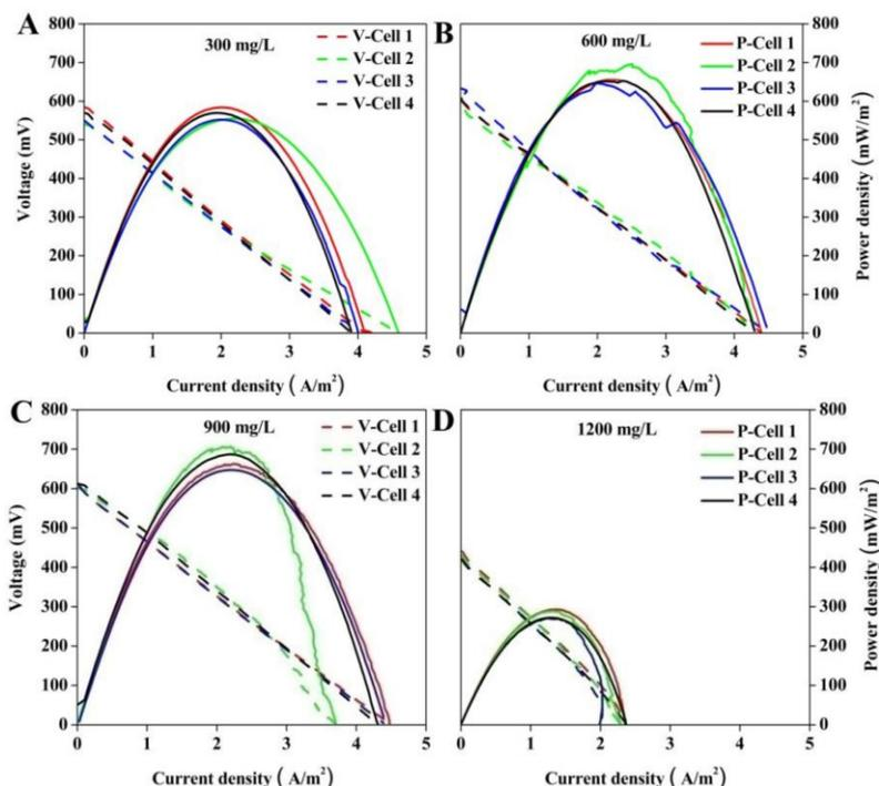
**Figure 3.** Polarization curves and power densities of the CSBES at different ammonia concentrations. (a): 300 mg/L; (b): 600 mg/L; (c): 900 mg/L; (d): 1200 mg/L.
