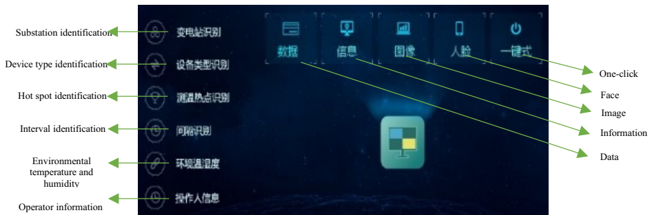
Figure 2. The functions intelligent data acquisition and analysis terminal.
