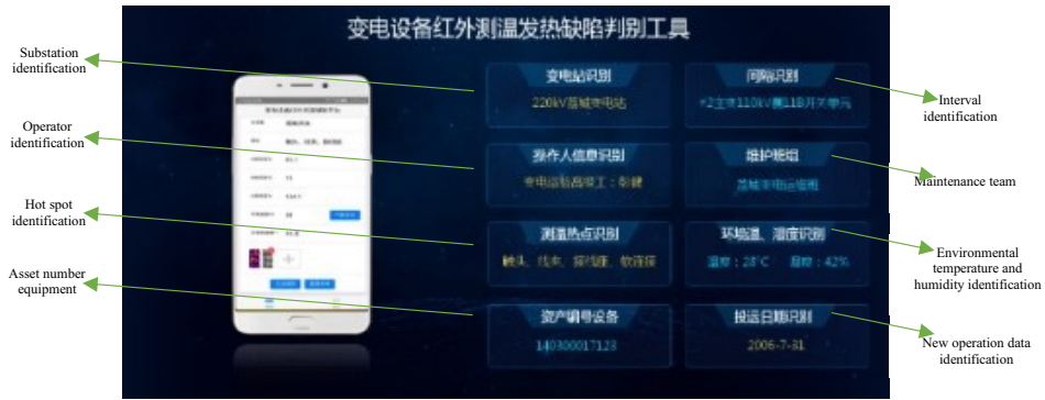
Figure 3. Schematic diagram of device heating defect discrimination interface in mobile phone client APP.
