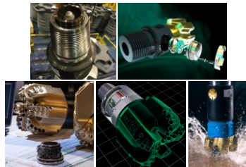
Figure 7. Measuring modules installed in bits.
