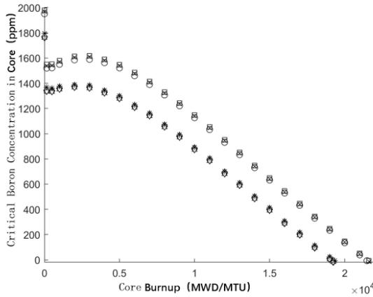
**Figure 1.** Variation of critical boron concentration with core burnup in each cycle.
