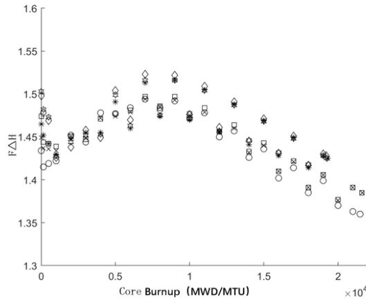
Figure 4. Variation of nuclear enthalpy rise hot channel factor with core burnup in each cycle.
