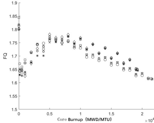
Figure 3. Variation of heat flux hot channel factor with core burnup in each cycle.
