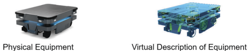
Figure 2. The physical equipment and its corresponding virtual representation.
