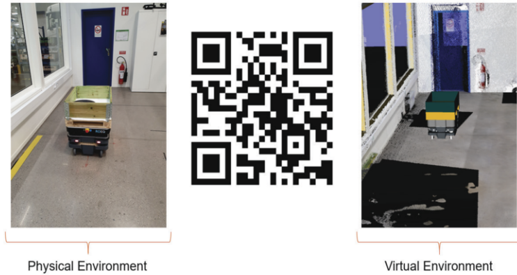
Figure 13. The QR code links to a video that demonstrates the real-time updates of the virtual environment based on changes in the physical environment.
