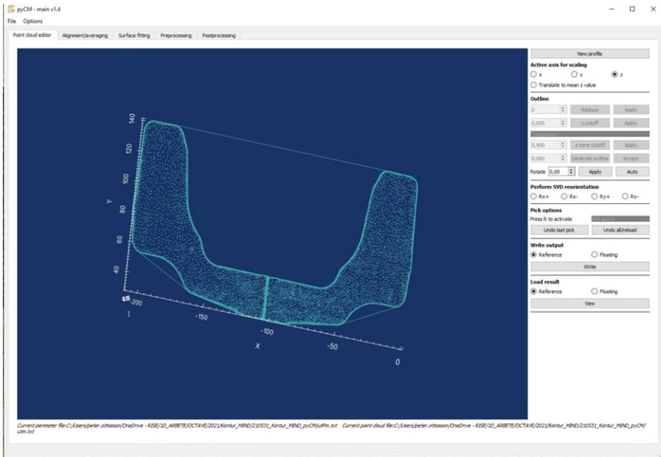
**Figure 13.** Outline visualized in PyCM generated from a point cloud using Alpha Shape Algorithm
