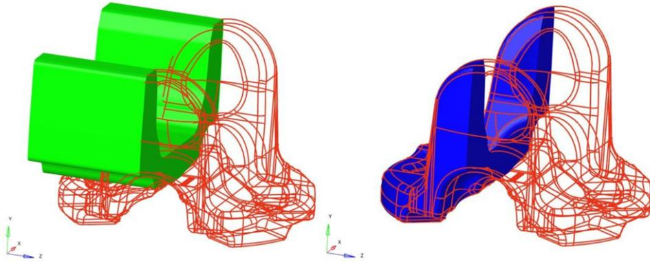
**Figure 9.** FE model based on extrusion of cut (left) and based on CAD-model (right)
