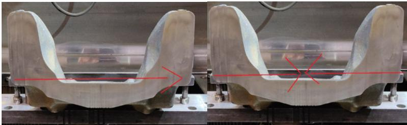
**Figure 3.** EDM with final cut at the end (left) and with final cut a final cut in the middle (right)
