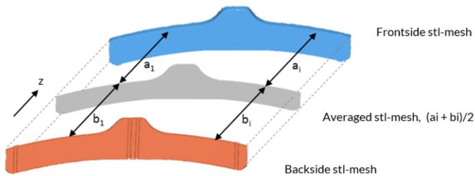
**Figure 7.** Calculation of average distortions
