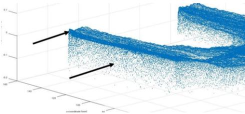
**Figure 6.** Removal of irrelevant datapoints from the stl models
