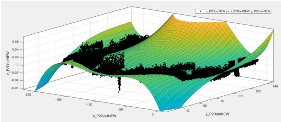
Figure 8. Polynomial surface of the cut based on averaged distortion vertex points
