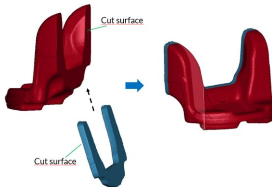
**Figure 5.** Manual positioning of the two stl models (blue and red) in order to align the cut surfaces
