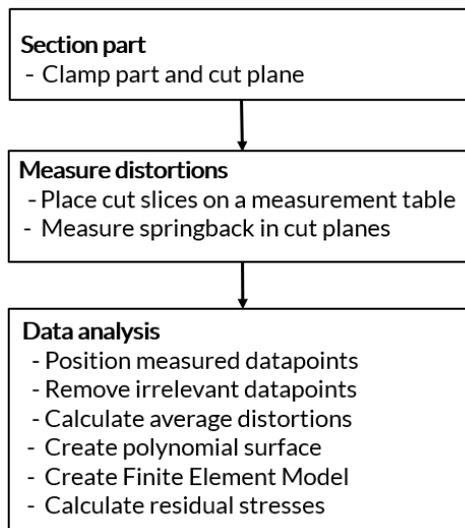
Figure 2. Procedures for prediction of bulk stresses in practice
