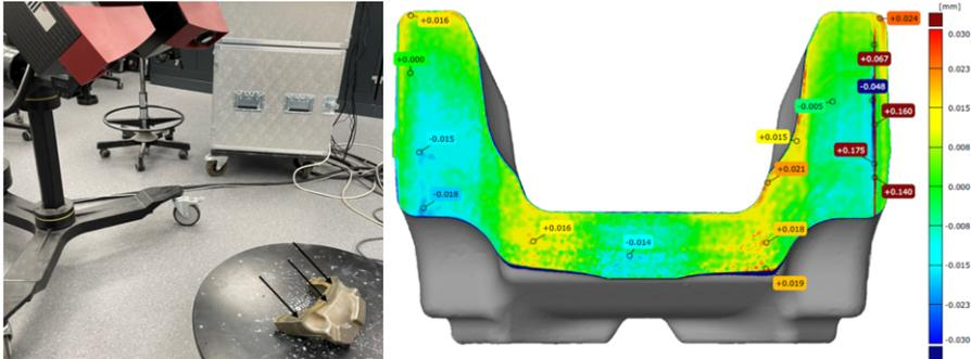
**Figure 4.** Measurement setup of out of plane distortions on cut section (left) and GOM measurement results from P1 cut (right)
