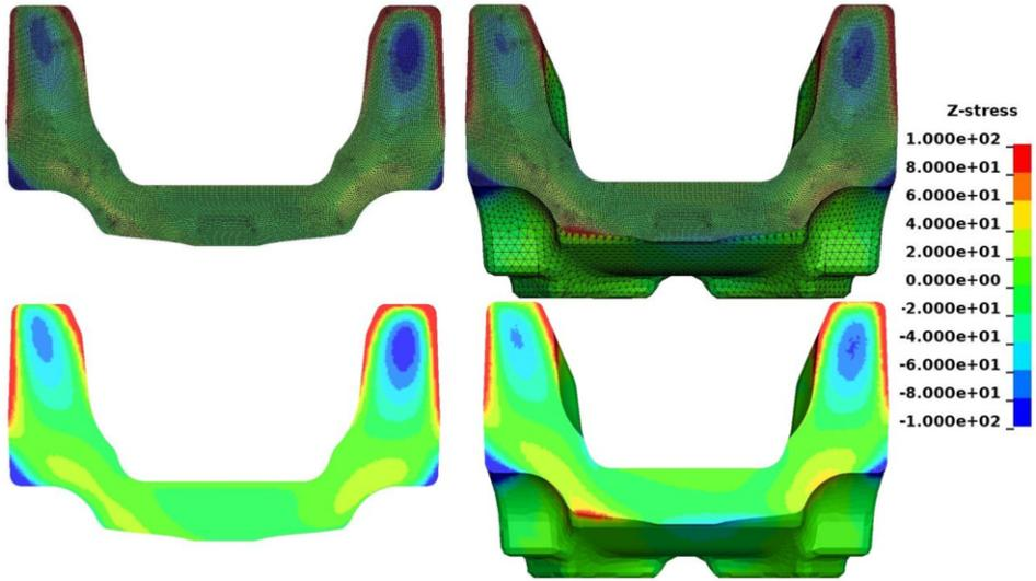
Figure 11. Out of plane stress results (z-stress) using extruded mesh (left) and Cad-model based mesh (right)
