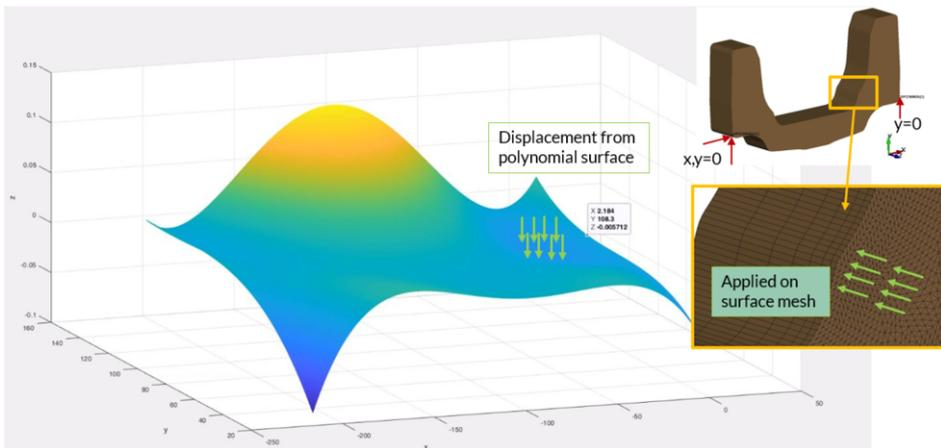
**Figure 10.** Boundary conditions for the Finite Element Analysis
