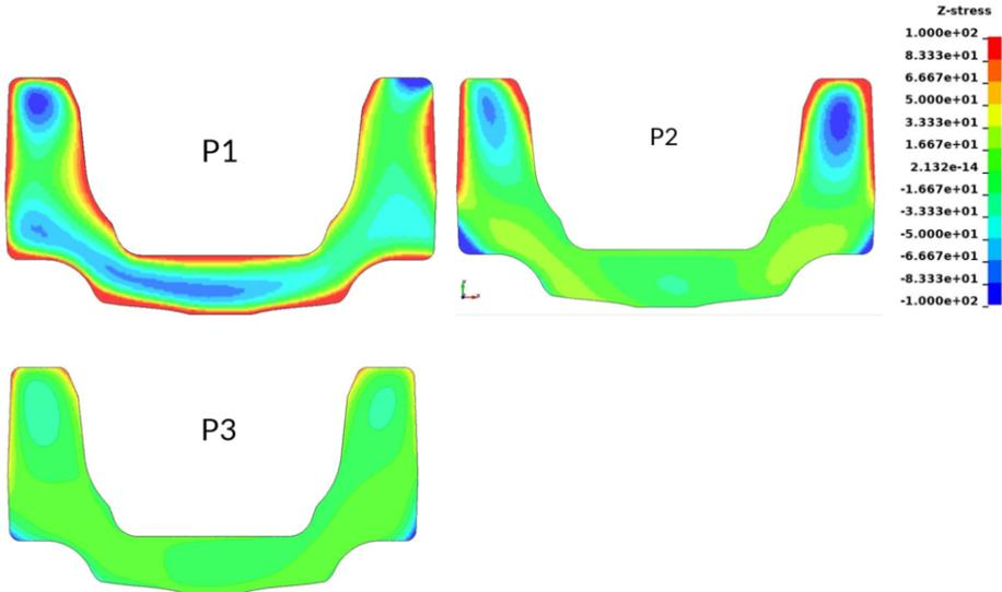
Figure 12. Out of plane stress results from P1 – P3 calculations
