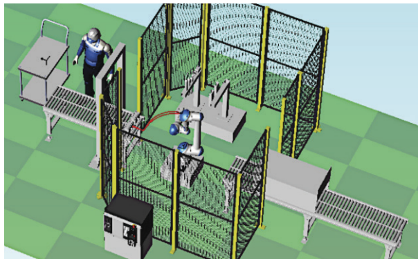
Figure 7: Concept for dispensing three sealants, mounting two lids, and curing in a tunnel [5].
