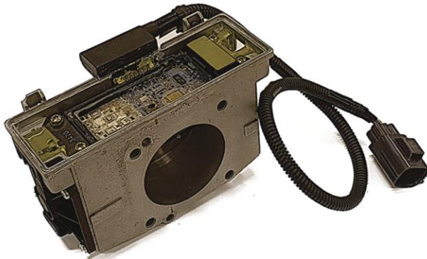
Figure 3. The core used in the case – An electro-mechanical throttle valve for car engines.
