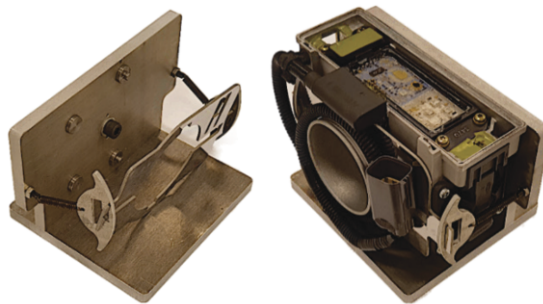
Figure 5: Carrier, without (left) and with mounted core (right).
