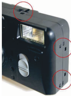
Figure 2. Camera design for automatic disassembly within remanufacturing [10].
