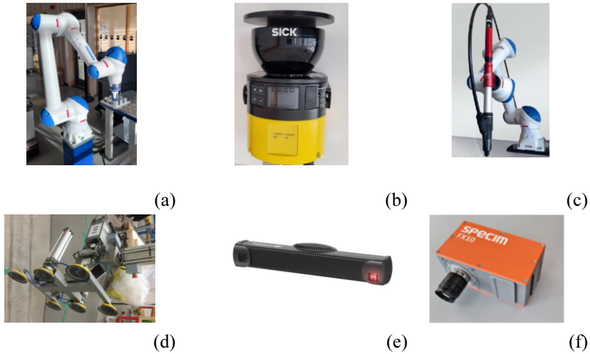
Figure 6: Hardware and peripheral equipment for the robotic window assembly cell: (a) Yaskawa Motoman collaborative robot, (b) SICK sensor, (c) Stöger automatic screwdriver RSX, (d) Vacuum gripper, (e) Photoneo vision sensor (PhoXi 3D Scanner), (f) Specim hyperspectral camera
