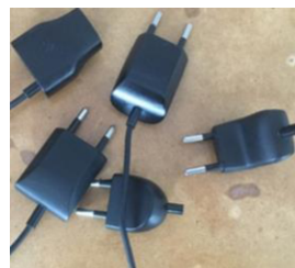
Figure 3. Hand-made prototypes of power supply cover.
