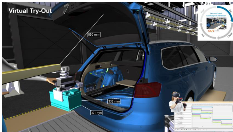
Figure 3. Human centric assembly cell validation. Model data is Courtesy of Volkswagen.
