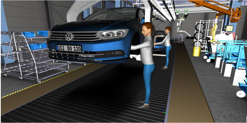
Figure 1. Experience assembly process with Digital Human Models. Model data is Courtesy of Volkswagen.
