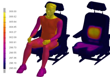
Figure 9. Temperature Distribution on Safran Seat done with ESI Interior Solution.
