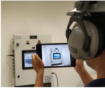
Figure 9. Using the Tablet to identify the panel and access the AR mode.
