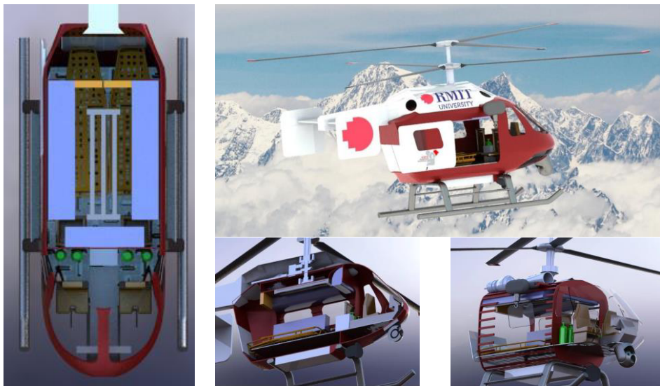
Figure 5. Final helicopter design configuration and layout.
