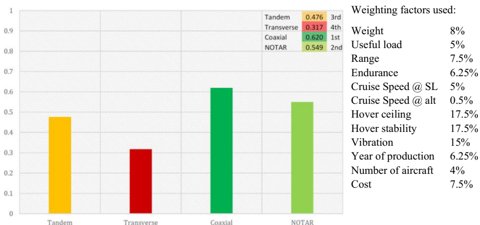
Figure 3. Rotor type selection.
