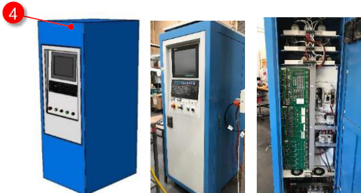
Figure 6. WEDM high-frequency pulse generator.
