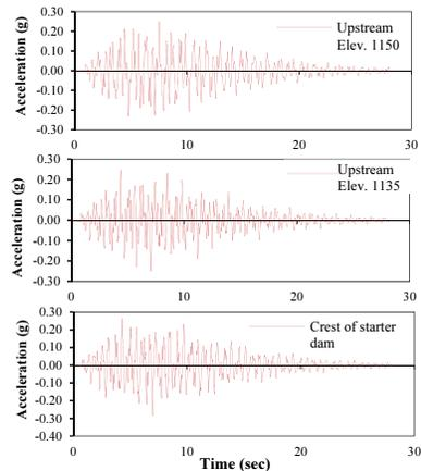
Figure 22. Acceleration time history at the crest of the starter dam and upstream dikes.
