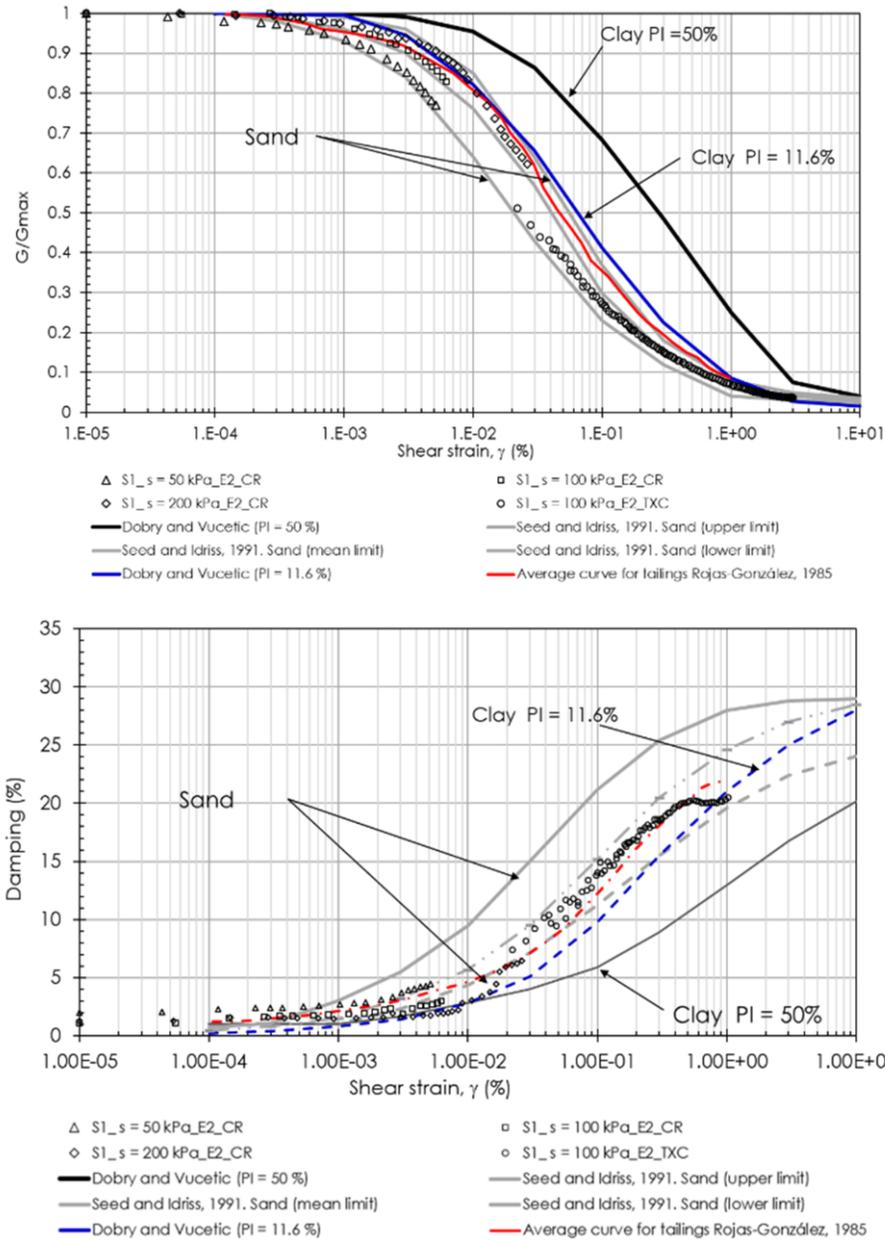
**Figure 11.** Curves of degradation of the shear modulus  $G/G_{max}$  and damping curves versus shear strain amplitude under different effective confining pressure in tailings.
