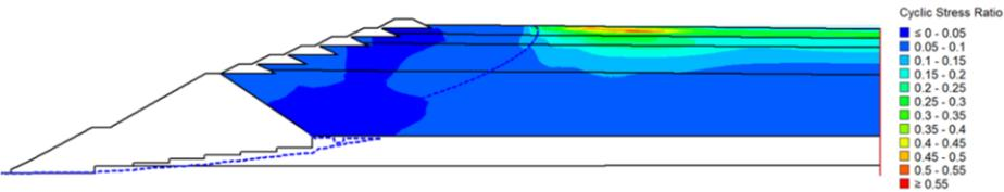
Figure 24. Cyclic stress ratio (CSR) contours computed in the numerical model.
