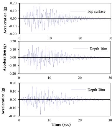
Figure 21. Acceleration time history at different depths in tailings.
