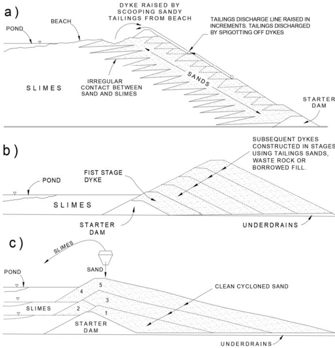
**Figure 2.** Methods of construction: a) Upstream, b) Downstream and c) Center-line (Figure modified from [5]).
