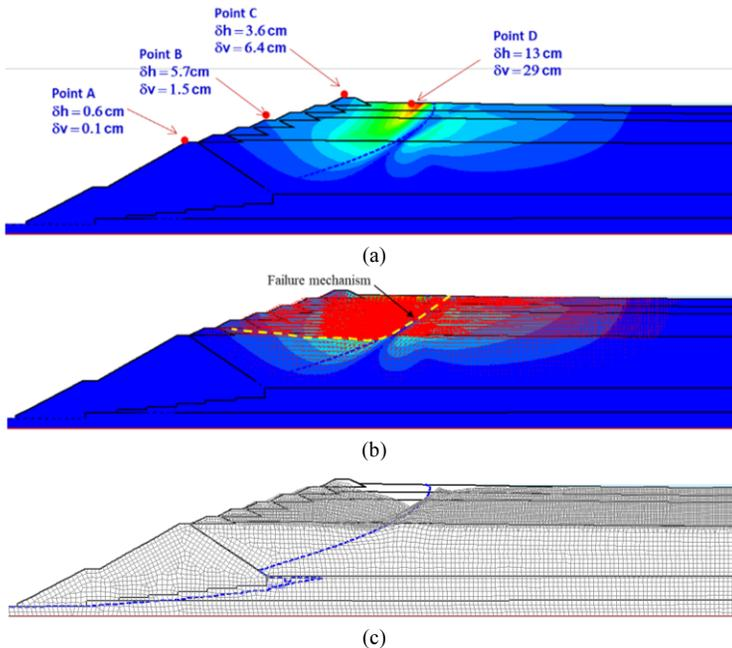
**Figure 25.** a) Post-earthquake deformations contours, b) Post-earthquake deformations in terms of displacement vectors b) and c) Distorted mesh of the model (50 times magnified).
