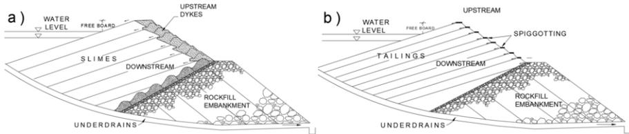
**Figure 3.** Scheme of upstream-downstream method with rockfill embankment: a) cyclone sand and b) spigotting (Figure modified from [8]).
