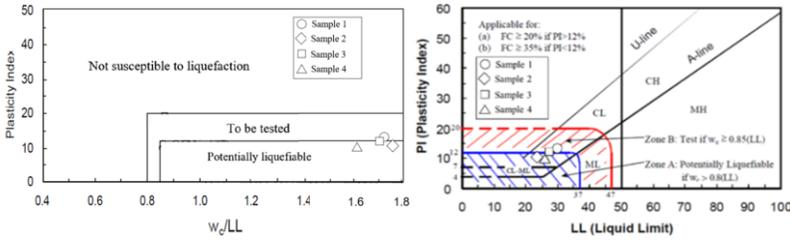
**Figure 13.** Assessment of the liquefaction susceptibility of the four samples of tailings: (a) Andrews and Martin criteria [14] and (b) Bray *et al.* criteria [15].
