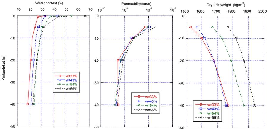
**Figure 10.** Simulation of the deposition process of tailings in situ: a) variation of water content, b) variation of permeability and c) variation of dry unit weight due to tailings deposition.
