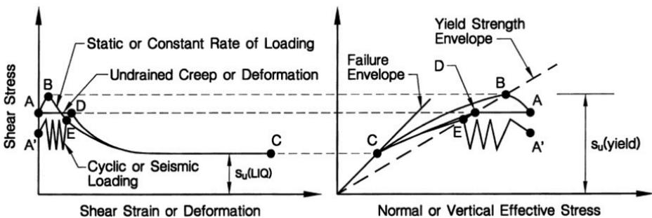
Figure 5. Flow Liquefaction behavior [23].
