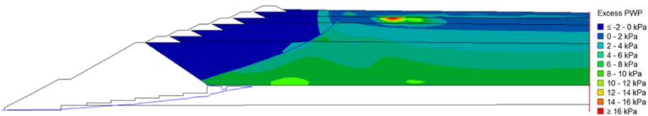
Figure 23. Excess pore pressures at the end of the earthquake.
