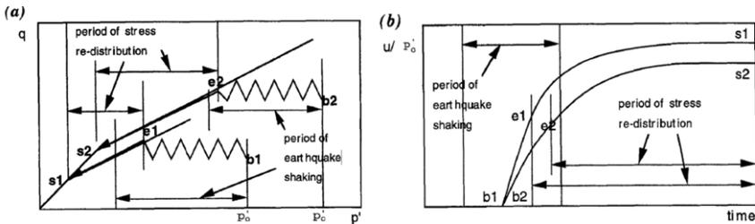
Figure 20. Delayed behavior caused by stress redistribution [43].
