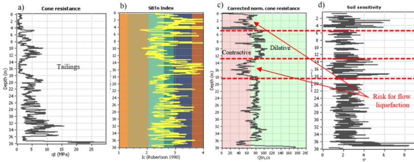
Figure 15. Cone penetration test results in tailing slimes.
