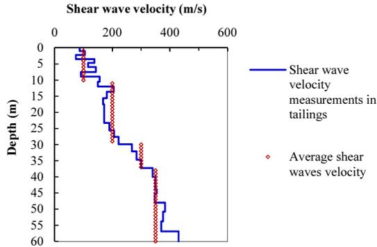
Figure 12. Shear wave velocities ( $V_s$ ) profile in tailings.
