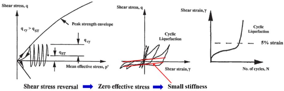
Figure 4. Cyclic (seismic) liquefaction behavior [18].
