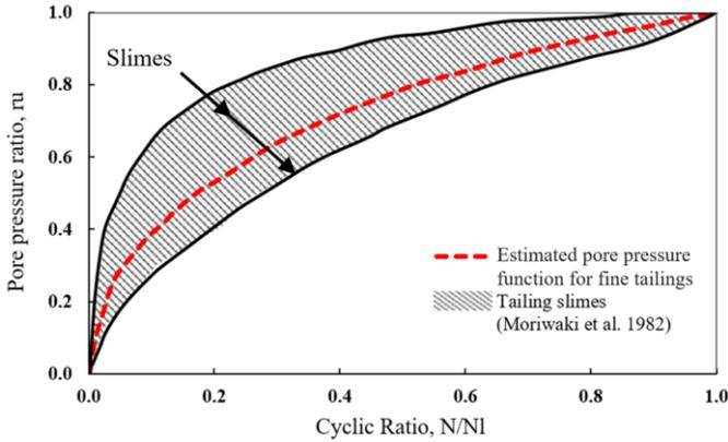
Figure 19. Pore pressure function for fine tailings.
