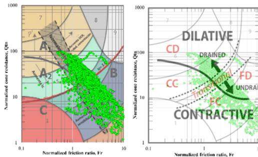
Figure 16. Evaluation of soil response in the CPT soil behavior chart.
