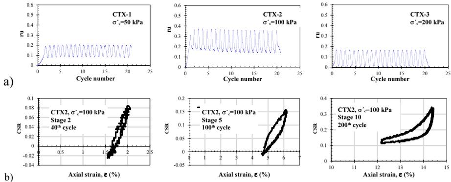
**Figure 14.** (a) Excess pore pressure ratio versus the number of loading cycles (10<sup>th</sup> stage) and (b) time histories of axial stress-strain hysteresis loops for different stages and cycle number from cyclic triaxial test CTX-2.
