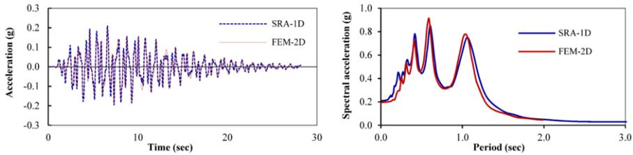
Figure 18. Comparison of acceleration record and response spectrum for SRA-1D and FEM-2D.
