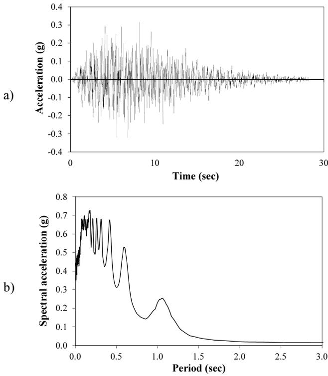
Figure 8. a) Input earthquake acceleration record and b) response spectra.
