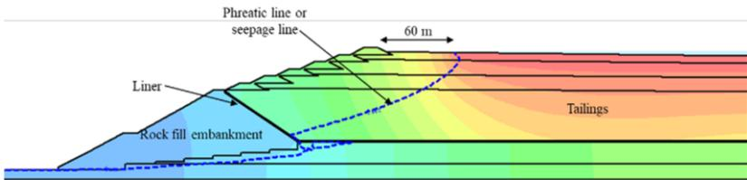
**Figure 17.** Seepage through the dam.
