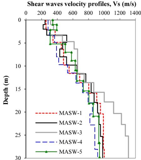
Figure 9. Shear wave velocity ( $V_s$ ) profiles in foundation.
