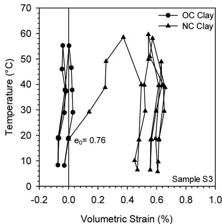
Figure 11. Volumetric response of NC and OC samples to thermal cycles.
