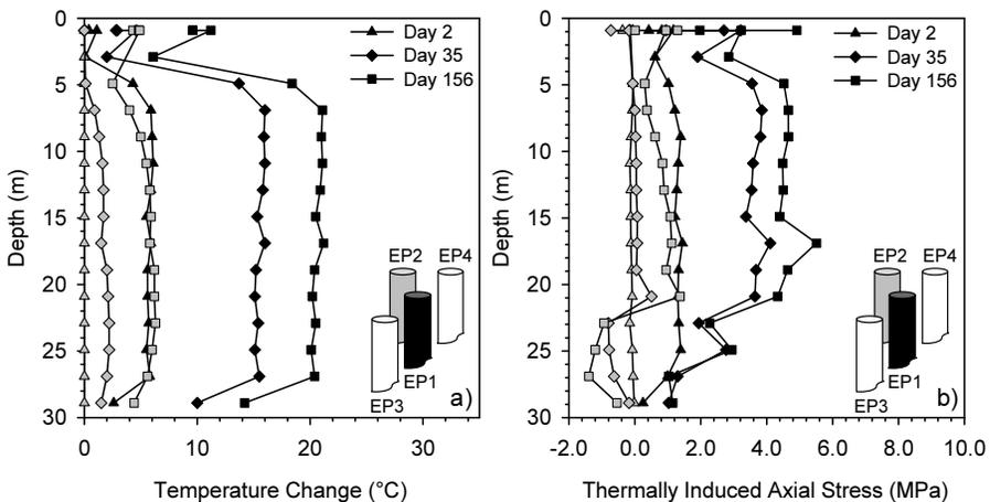
**Figure 4.** a) Temperature changes b) Thermally induced axial stresses along EP1 and EP2 due to geothermal operation of EP1.
