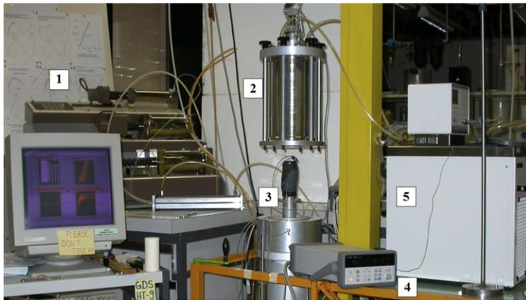
**Figure 8.** Thermal triaxial testing apparatus (1: GDS Controller, 2: Triaxial Cell, 3: Thermocouple, 4: Multiplexer, 5: Heating bath).
