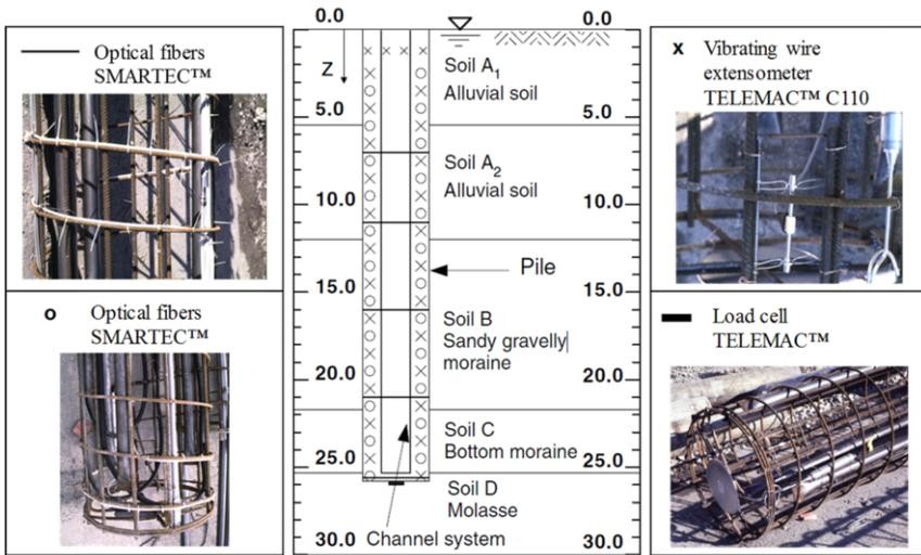
Figure 1. Soil profile at the site and sensors along the test pile (Test Site-1).
