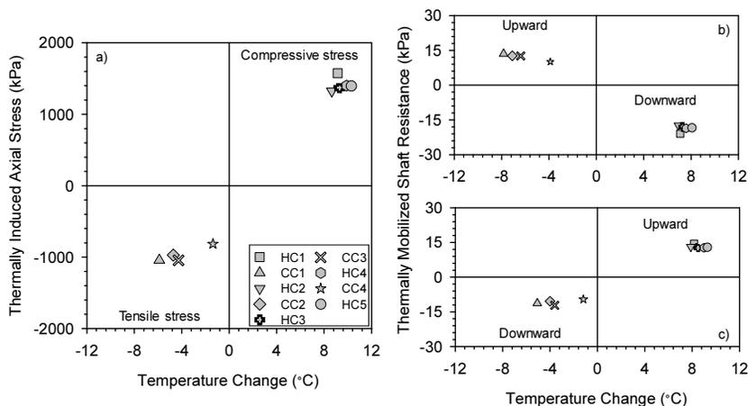
**Figure 7.** a) Thermally induced axial stress at null point; Mobilized shaft resistance at b) clay layer, c) sand layer due to thermal cycles.
