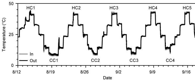
**Figure 6.** Circulating fluid temperature in the heat exchanger tubes embedded in the test pile.
