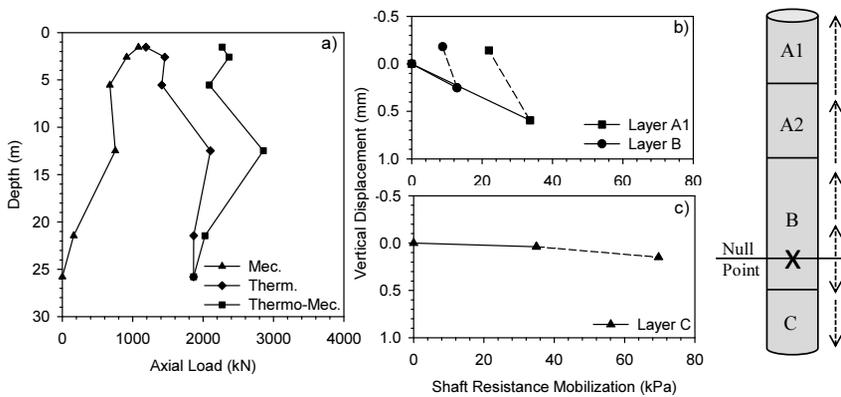
Figure 2. a) Mechanical, thermal and thermo-mechanical loads and b,c) shaft resistance mobilization along the test pile.
