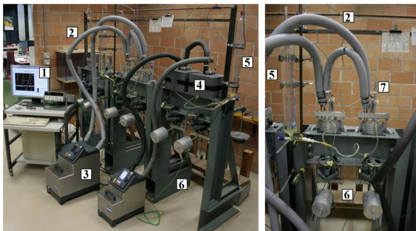
**Figure 10.** Thermal oedometer device (1: Acquisition system, 2: Tubes with circulating water, 3: Heater, 4: Insulation, 5: Water supplier, 6: Thermocouple, 7: LVDT).
