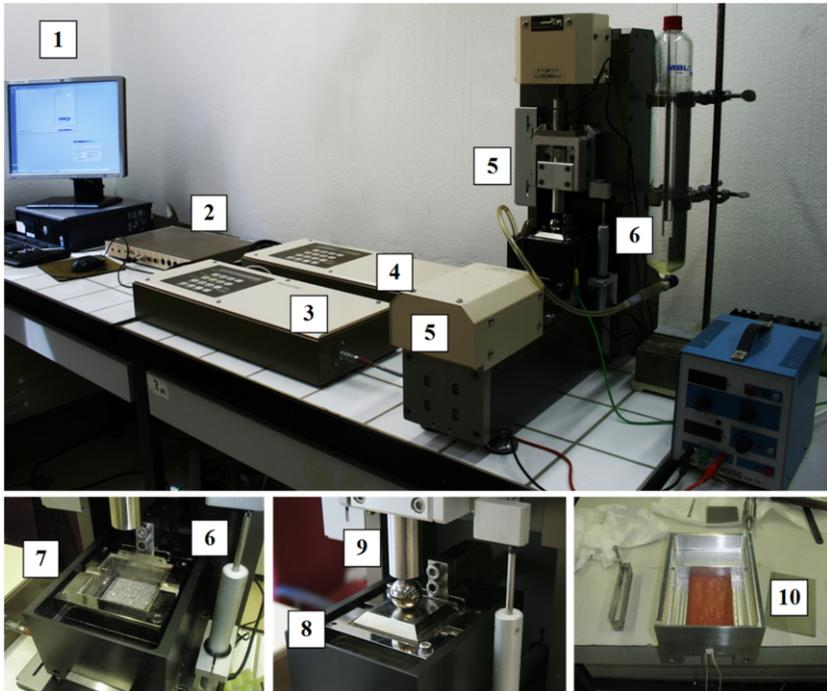
**Figure 13.** Thermal interface shear testing apparatus (1: GDSLAB software control, 2: LVDT Acquisition, 3: Normal actuator, 4: Horizontal actuator, 5: Load cells, 6: LVDT, 7: Specimen placement, 8: Top cap, 9: Axial piston, 10: Heating system).
