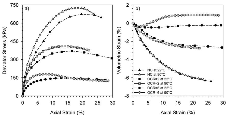
**Figure 9.** Drained triaxial tests at ambient (22°C) and elevated (90°C) temperatures
