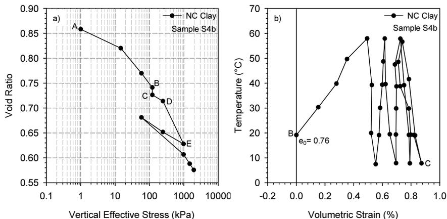
Figure 12. Effect of thermal cycles a) on the oedometer curve, b) on volumetric strain
