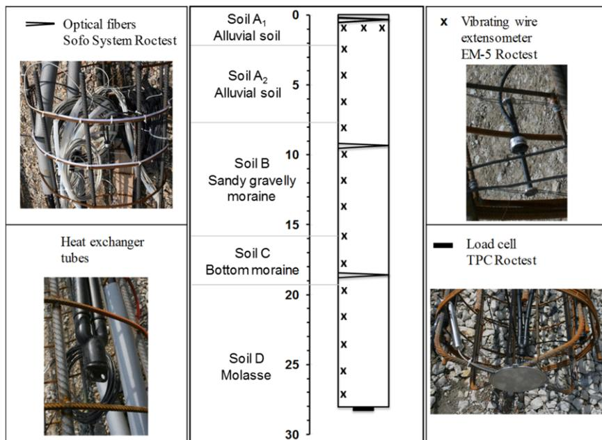
Figure 3. Soil profile at the site and sensors along the test piles.
