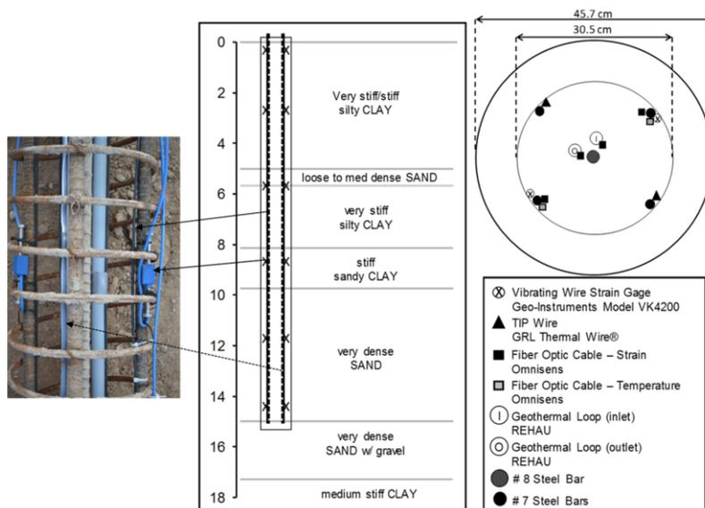
Figure 5. Soil profile at the site and sensors along the test pile.
