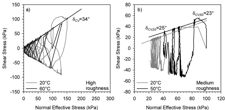
**Figure 14.** CNS tests on a) Sand-concrete interface (high roughness), b) Clay-concrete interface (medium roughness).
