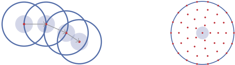
a) Illustration of footsteps of agent i . The circles (blue) indicate the actual step radius \lambda_i and the shaded area (blue) represents the agent torso of radius r_p .
