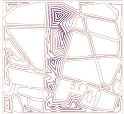
b) Distance function \hat{d}_\Omega which gives the minimal distance to the nearest obstacle.
