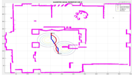
Figure 6. Wheelchair trajectory respecting the social restrictions theoretically in Matlab, in a museum and with objective the central museum
