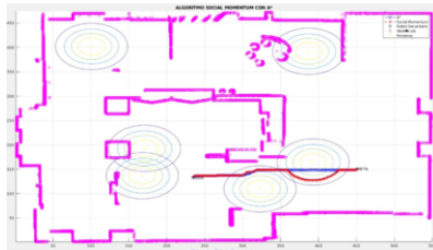
Figure 4. Wheelchair trajectory respecting the social restrictions theoretically in Matlab, in a museum and with objective the entrance
