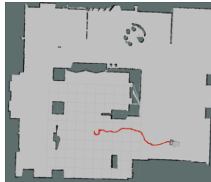
Figure 5. Wheelchair trajectory respecting the social restrictions practically in RViz, in a museum and with objective the entrance
