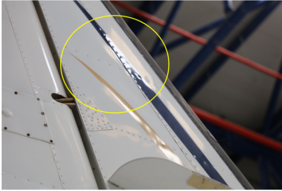
Figure 2. The gaps could be due to lose fasteners in edge of skin lap. Defect can easily be missed if not inspected standing on a work stand. The light plays an important role in damage detection. Photo taken at Abu Dhabi Polytechnic Hangar.
