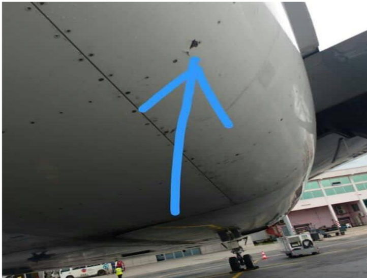
Figure 6. Example of a rare defect: Gunshot Damage of an A330-300 hit by a bullet in Congo on April 11 th , 2020.
