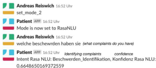
Figure 3. Slack integration of the anamnesis chatbot. User chooses Rasa NLU as a classifier. Input sentence contains an intentional spelling mistake and the chatbot returns the classified intent and its confidence value.
