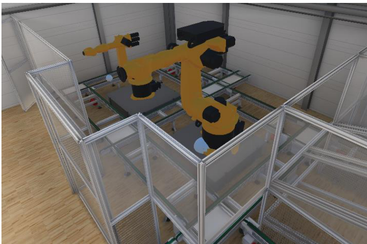
Figure 7. Graphical model for virtual commissioning
