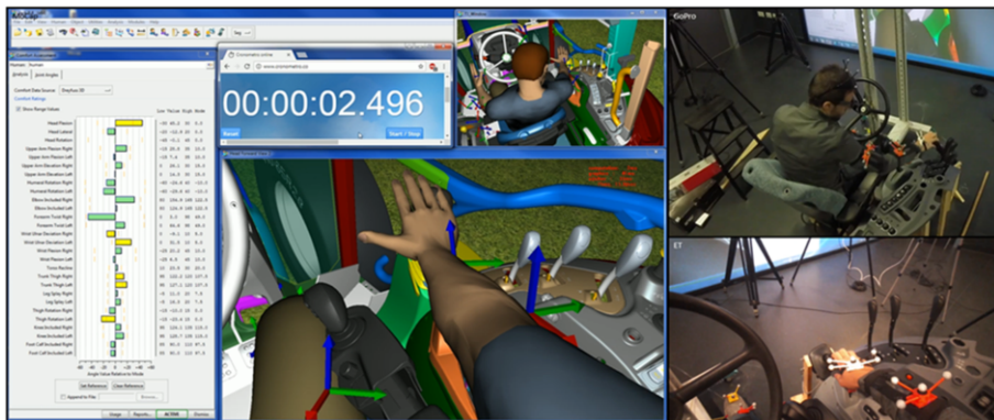
Figure 3. Results about physical stress by Dreyfuss 3D data for a specific posture
