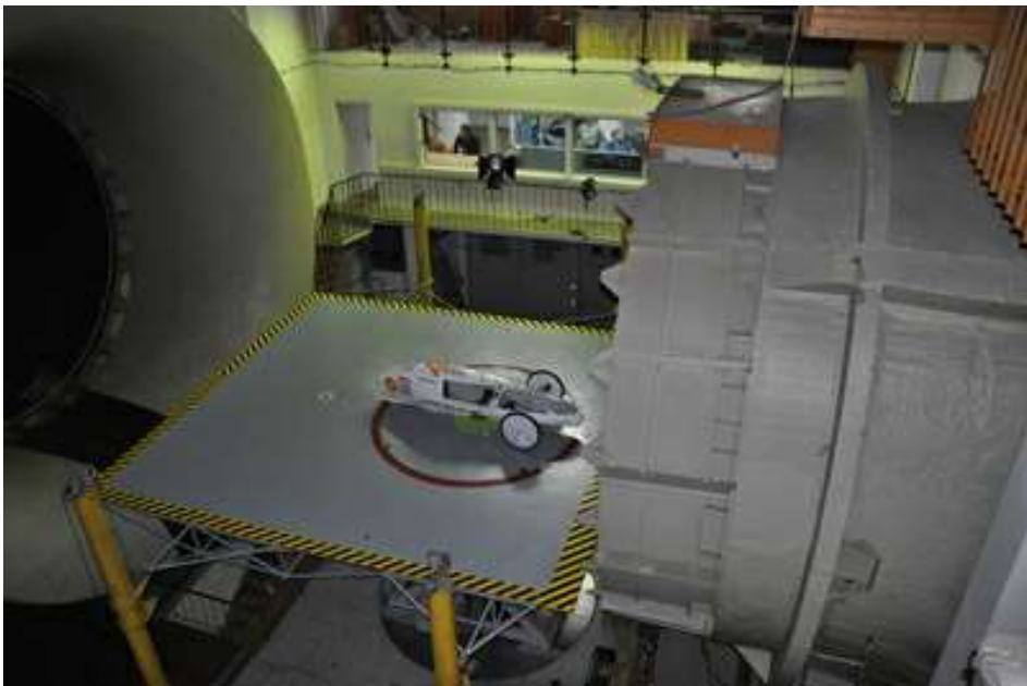
Figure 7. Verification of aerodynamical characteristic in wind tunnel.
