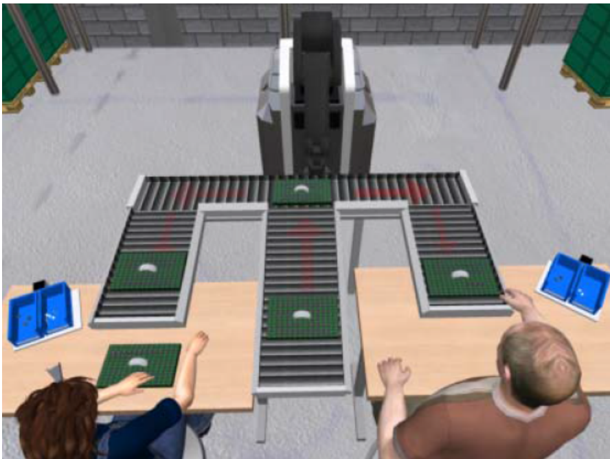
Figure 4. Third scenario of the human-robot collaboration workplace for up to 2 workers, with passive roll-based conveyor band.
