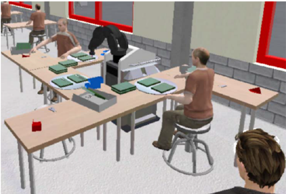
Figure 3. Second scenario of the human-robot collaboration workplace for up to 3 workers with 2 split assembly fields on the rotary plate. The control rack is arranged in an angle of 90° to the right of the worker.
