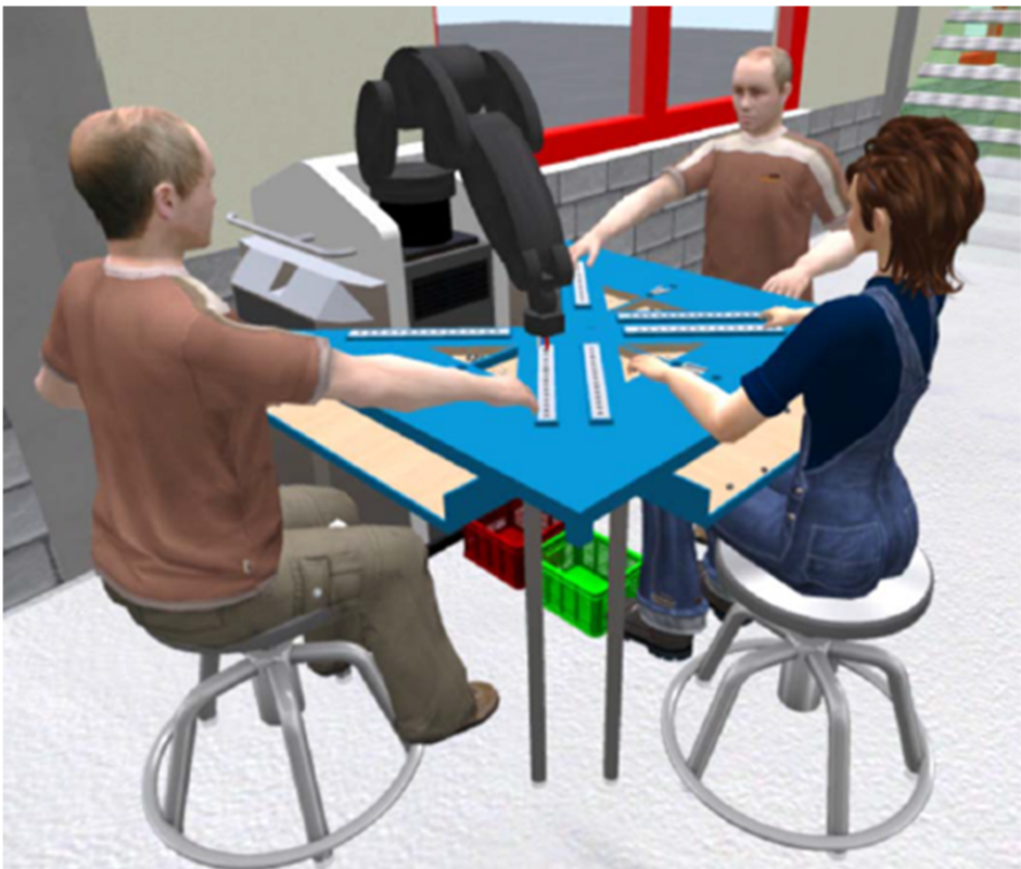
Figure 2. First scenario of the human-robot collaboration workplace for up to 3 workers, designed with V-shaped racks for positioning of the valve elements.
