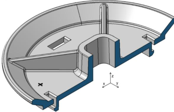
**Figure 3.** CAD: Section view of one V-belt pulley half.
