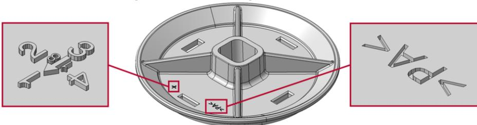
Figure 6. CAD: Integrated part markings on the V-belt pulley.
