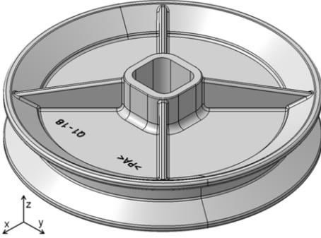
**Figure 7.** Isometric view of the adapted V-belt pulley.
