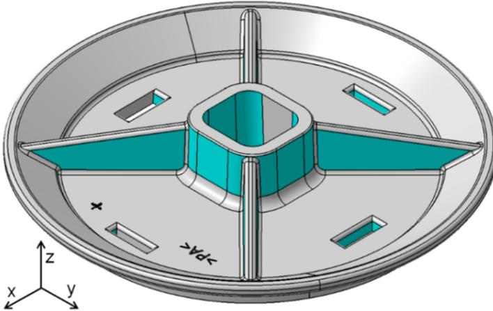
Figure 5. CAD: V-belt pulley with highlighted draft angles.
