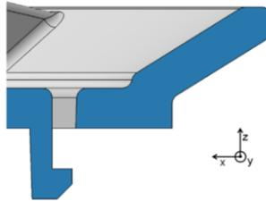
**Figure 4.** CAD: Section view of snap hook and belt guide.
