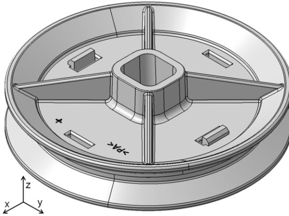
**Figure 2.** CAD: Isometric view of the assembled V-belt pulley (based on [11]).
