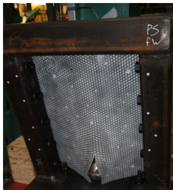
Figure 1: Raking damage tests: Mild Steel specimen is subjected to a lateral impact load. Deformation is recorded with DIC (Haag et al. , 2017).
