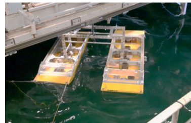
Figure 4: Scaled test of the float-over concept with flexible topside (Dessi et al. , 2017b)
