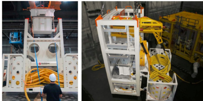
Figure 4.8: Subsea step-down transformer modules with electrical flying leads during assembly (left) and during system testing (right) (Hjelmeland et al. , 2017)
