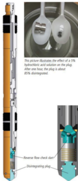
Figure 3.6: Gas lift valve with HSDM (Carrejo et al., 2015)
