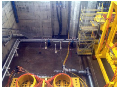
Figure 4.4: Slug test loop arrangement (Bibet et al. , 2016)
