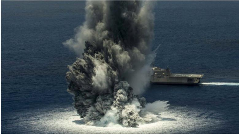
Figure 12: USS Jackson (LCS 6) undergoing shot 1 of 3 full scale shock trial.
