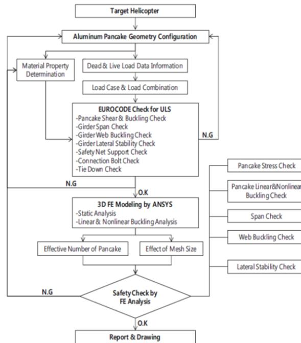
Figure 19: Flow chart showing the design process of an aluminium helideck structure
