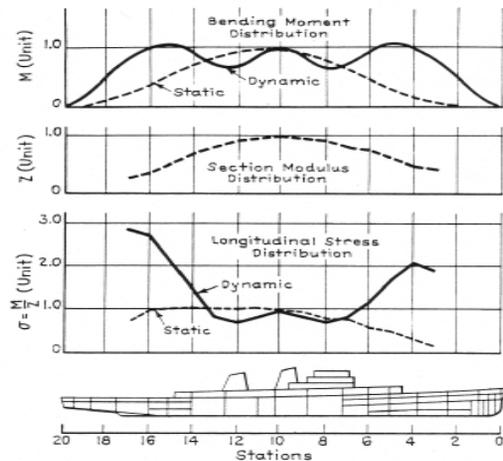
Figure 10: Illustration of load curves under static and dynamic response, (after Kiel 1961),
