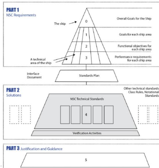
Figure 8: Arrangement of the Naval Ship Code
