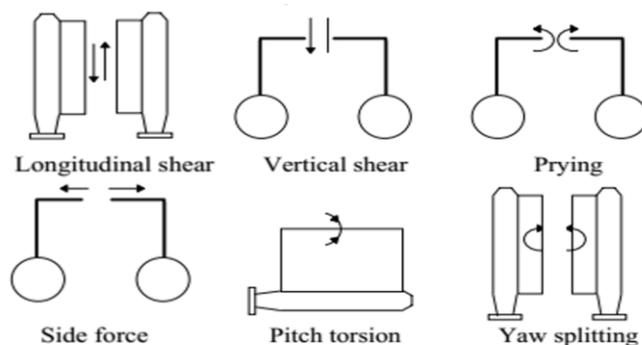
Figure 17: Considered Design Loads on SWATH Hull Structure
