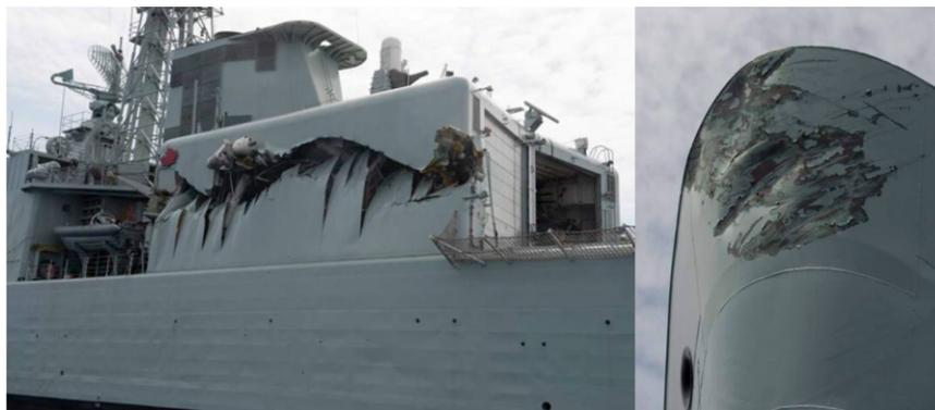
Figure 11: On left: collision damage to aluminium superstructure. On right: only slight collision damage to the steel (naval) ship bow responsible for destroying the al superstructure.
