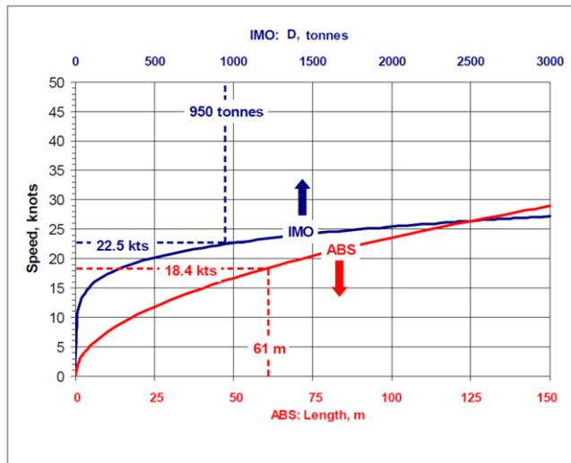
Figure 6: IMO and ABS Definitions of High Speed Craft (SSC 2005)
