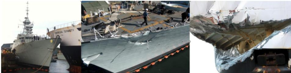
Figure 13: On left, collision between merchant and warship. Center: Warship damage. Right: Merchant damage.
