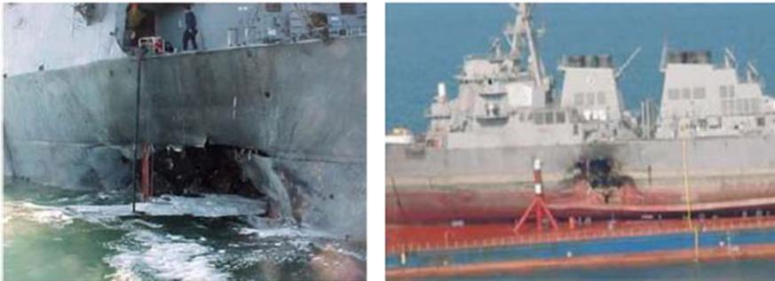
Figure 9: USS Cole following contact air blast detonation showing the protection against crack propagation afforded by the ~2m wide high strength steel sheer strake<sup>1</sup>
