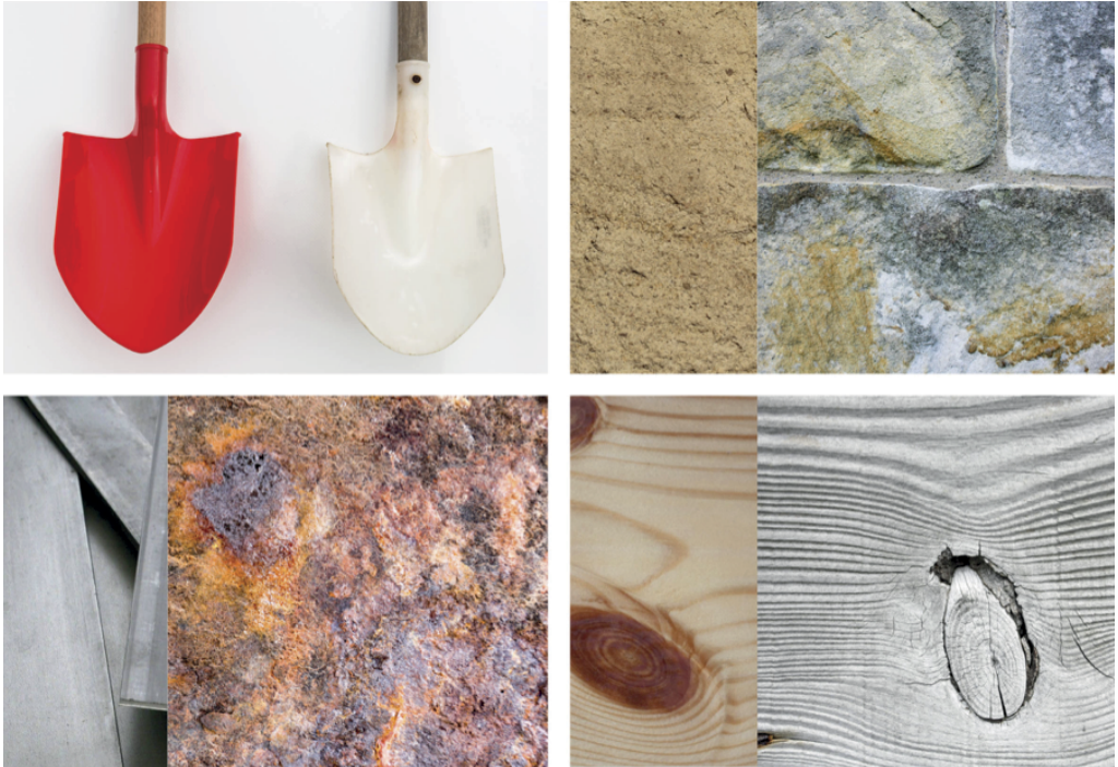
Figure 1. Materials change (clockwise from top left): a plastic spade is severely faded by sunlight (despite it being designed for outdoor use); sandstone develops a rich patina of lichen; wood has lost colour but the surface texture is accentuated after exposure to sunlight and salt from the sea; mild steel reacts with oxygen and water to produce beautiful but fragile rust. In each case the new material is on the left. Except for the spade, the new and old materials are similar but not identical samples.
