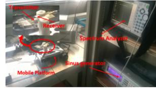
**Figure 6.** Setup measurement platform for Ultrasonic propagation analysis
